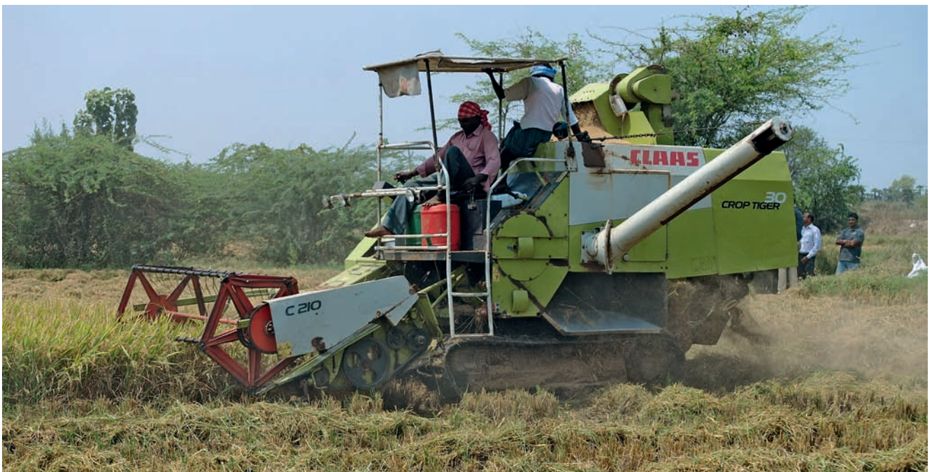
Model Crop Tiger in India, developed by Claas. It was originally designed for the rice harvest. Thanks to further developments, it now has the ability to tackle grain as well.
